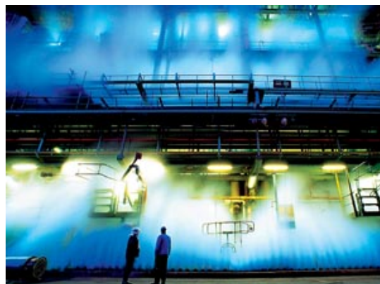
A steam/ammonia curtain immediately neutralizes hazardous gases in the event of an accidental release.
