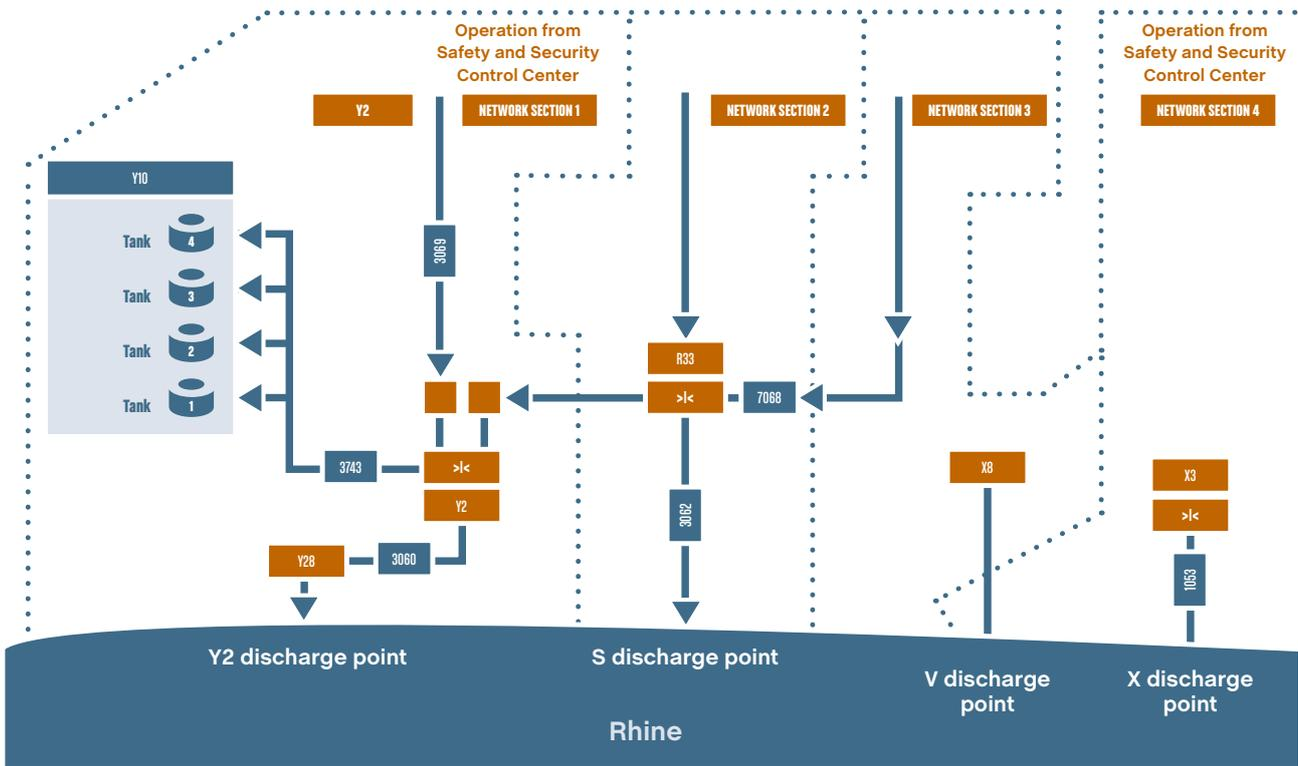
Fig. 2: Sewer systems for cooling water and organically uncontaminated water
