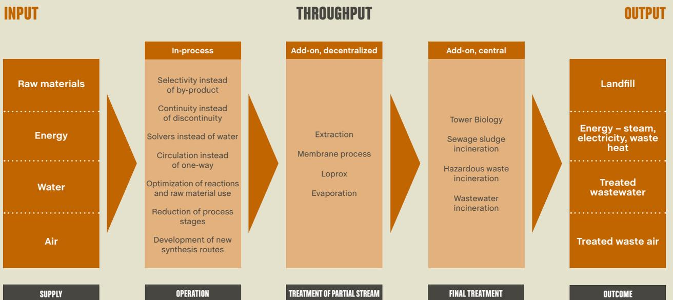
Fig. 3: Decentralized processes for the initial treatment of solid waste, wastewater and waste air
